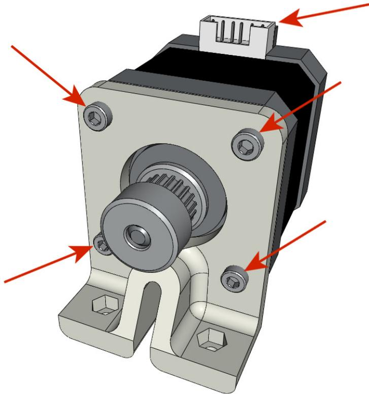
**Attention:** The illustration shows a motor support provided for a belt of 200mm but the mounting is the same with a motor support provided for a belt of 220mm.
